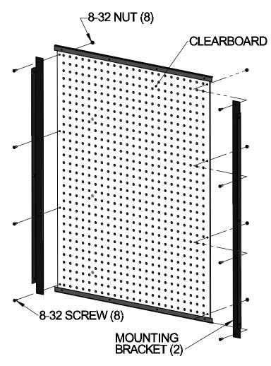
1. Peel back the protective covering on one side of the ClearBoard and attach a Mounting Bracket by loosely installing the 8-32 hardware as shown. Bracket should be on same side of the plastic pegboard as the attached metal brace, with screws entering from this side and the nuts against the pegboard. Don't tighten yet. Repeat for the other side.
