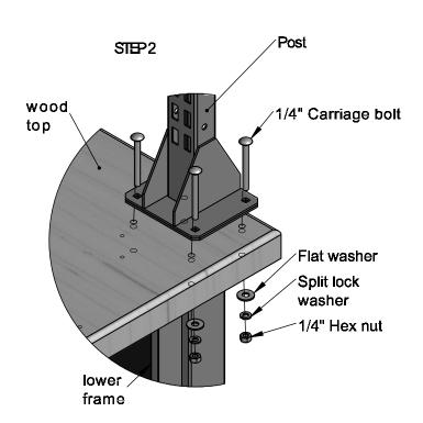
2) With wood top in position and secured on the lower frame, attach each post to the WorkTable by loosely installing four each: 1/4" carriage bolts, flat washers, split lock washers, and 1/4" Hex nuts.
