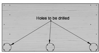
1) Notice the 12 larger partially-drilled holes on the underside of the table. With wood top unattached to the WorkTable carefully complete the 12 holes shown with a 9/32" drill bit. Be sure drill is held straight, and to avoid splintering DO NOT drill with excessive force.
