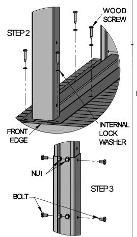
3) The total height of this unit is adjustable from 25.5" to 37" (without casters). Expand the leg frames to your desired height and install four (4) 1/4" bolts in each leg from the outside as shown, threading the nuts from the inside.
