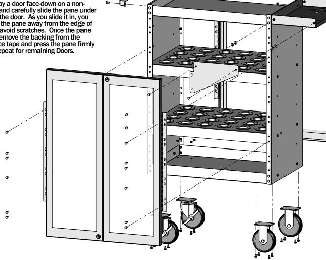
**6.** Loosely affix the Tray Brackets to the Sides as shown. Mount Side Trav. placing 2 washers between Tray and Bracket for each of the 4 bolts shown. Install nuts and bolts in the 2 remaining Tray holes (against the Side). Install the handle on the opposite end. Fully tighten all hardware.
