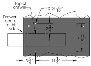
Installation on this product requires drilling 8 holes (4 on each side) per the above sketch.
