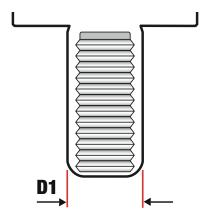
VDI toolholders come in many different shapes and sizes. One distinctive feature is the shaft is serrated on one side as shown in the illustration.
