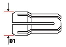
DA is short for double angle which refers to the two short angles which hold the tool in place.
