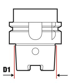
HSK's have a short hollow taper and we have identified 6 different styles.
