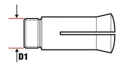
C/3J/R8 collets have a narrow cylindrical body, a short tapered head, and are threaded at one end.
