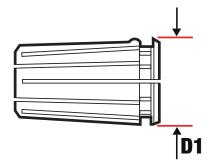
TG collets, short for tremendous grip, have a single shallow-angled taper similar to ER/RD/DR collets, but the difference between the types can be discerned by comparing dimensions.
