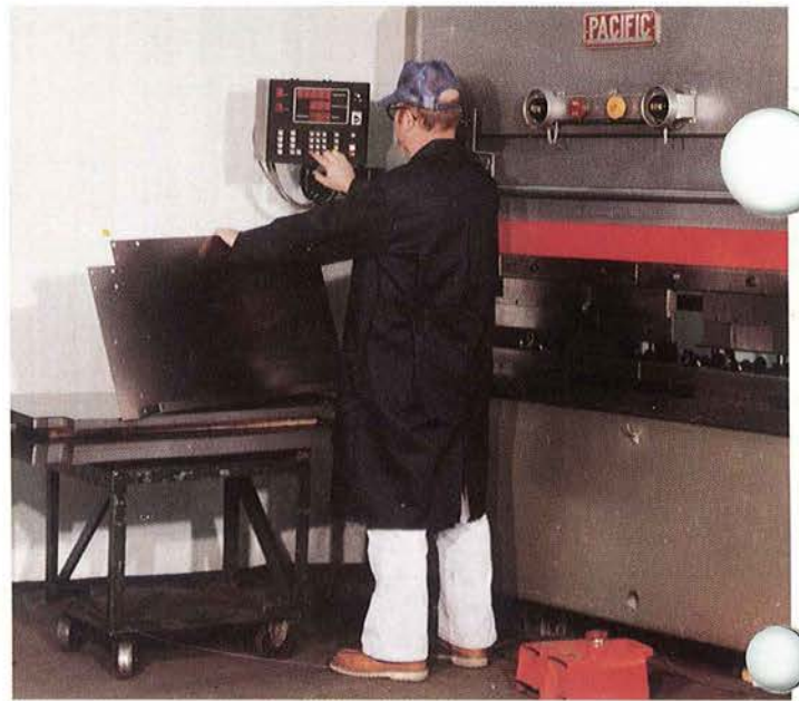
Computerized press brake operations for accuracy.
