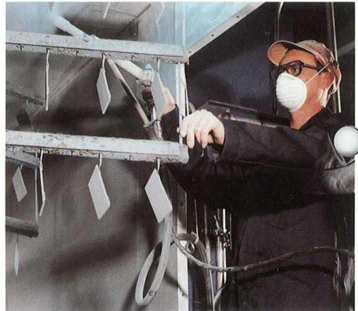
Electro-static plastic powder painting. Non-Polluting, tough-durable finish on all products.
